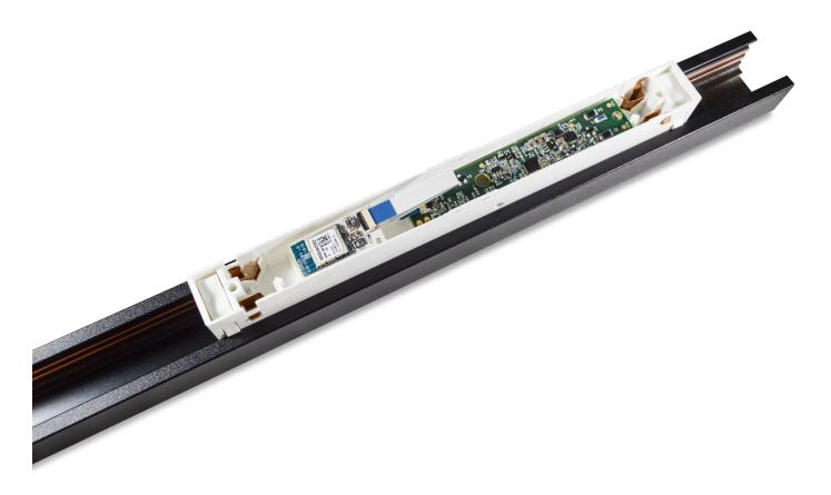
Figure 1: Xicato Miniature Driver (XMD) with Xicato GalaXi Card Bluetooth dongle shown inside a standard Stucchi® track adapter.
